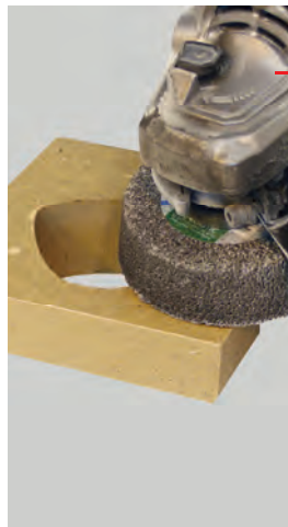
grinding the adhesive surfaces
