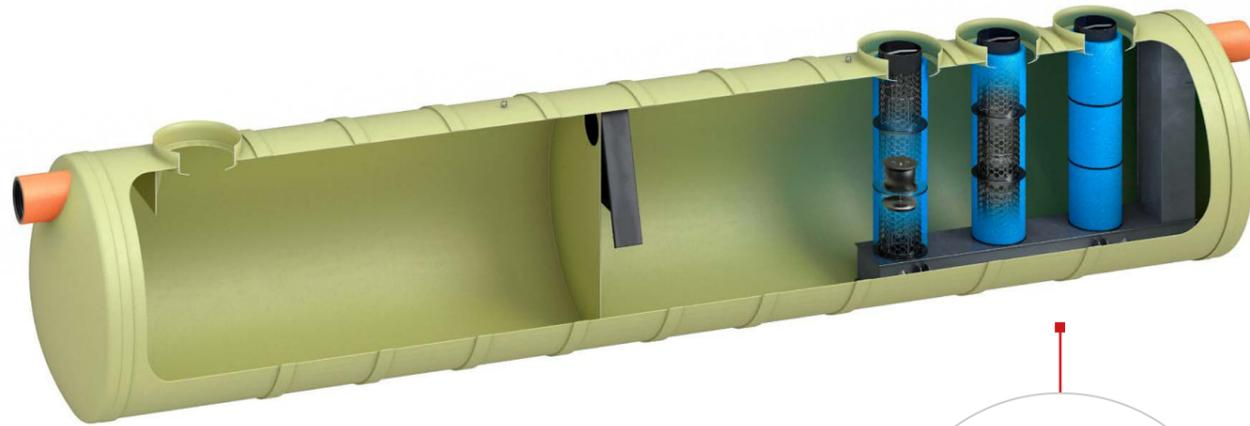
The new coalescence unit contains PU (polyurethane) foam to provide superior coalesce efficiency in the three segments. Each PU segment is firmly attached to the PE basket. PU segments are easy-to-clean and, if necessary, replace.
